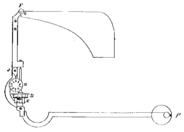
Then place the point of the tracer, F, upon any given point, say Q, of the outline of the figure to be measured, and either adjust the wheels to their respective zeros or take a first reading where they happen to stand: follow the outline of the figure carefully with the tracer point, moving in the direction taken by the hands of a watch, returning to the starting point Q; then the index must be read.
