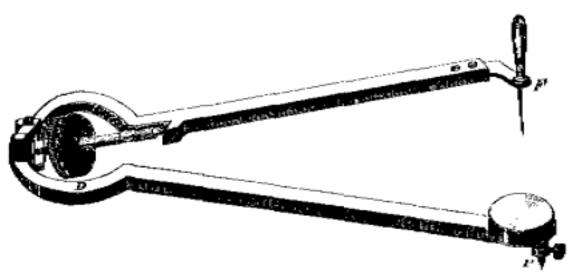
No. r represents the Planimeter as designed to measure the area in square inches and decimals of a square inch, in its simplest form—it having but one wheel; the figures on this wheel represent units, the intermediate graduations, tenths, and the vernier gives the hundredths. Limit of measurement, 10 square inches.
