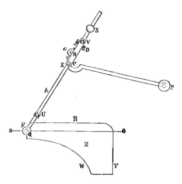
It will be noticed that in this instrument the arm A, carrying the tracer point, is capable of being varied in length. This is for the purpose of registering the result in various denominations of measurement, the value of which are well known, such for instance as square millimeters, square feet, square inches, etc., etc. The sliding bar A, is graduated with several vertical lines, alongside of which is engraved the particular value given to the smallest
